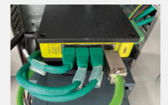
Online remote Access Integrated modem to enable remote access for Pujolàs technical service. Usable through either cable or Wi-Fi connection.
